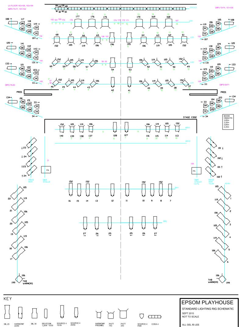
ALL GEL IS LEE FOH RIG IS FIXED POSITION AND CANNOT BE MOVED CH1-6 AND 17-22 ARE FIXED FOCUS / COLOUR
